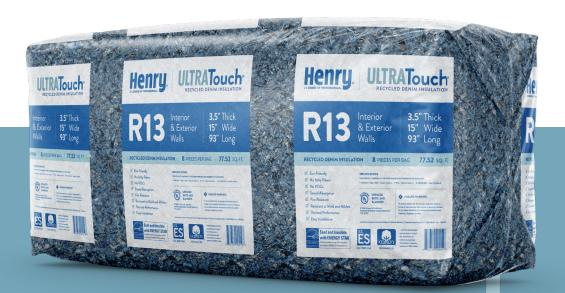
UltraTouch™ Recycled Denim Insulation is easy to install and does not require a certified installer. Wherever insulation is installed in a building, it is very important that it fits snugly on all sides. If the insulation is too long for a space, cut it to the correct size. If it is too short, cut a piece to fill the void. For our unfaced batts, simply friction fit the insulation into the cavities.
